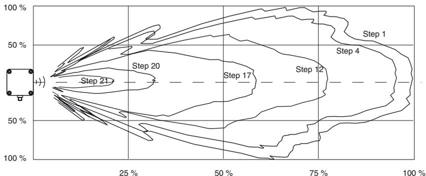
**Sensitivity adjustment for suppression of disturbing targets**
